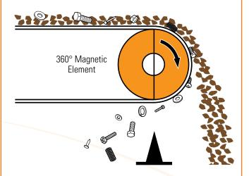
Ferrous metals are discharged conveniently underneath the end of the conveyor
